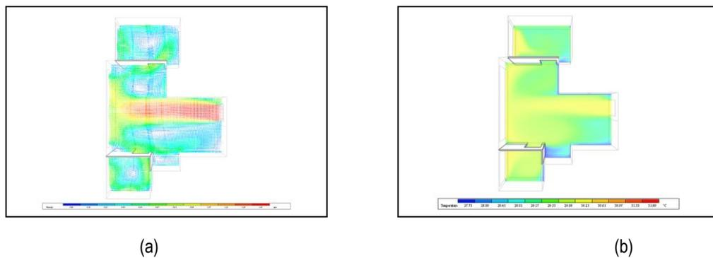
Fig. 8. (a) Air Velocity patterns (West Unit) simulation results; (b) Air Temperature Contours (West Unit)
