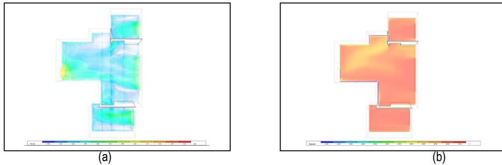
Fig. 7. (a) Air Velocity patterns (East Unit) simulation results; (b) Air Temperature Contours (East Unit)
