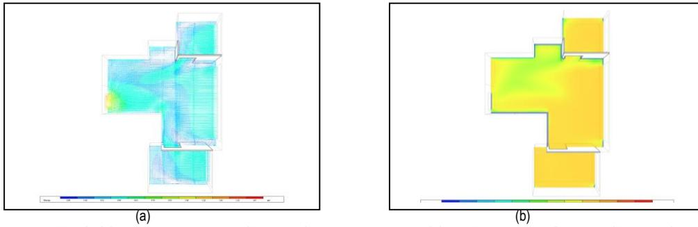
Fig. 9. (a) Air Velocity patterns (East Unit) simulation results; (b) Air Temperature Contours (East Unit)
