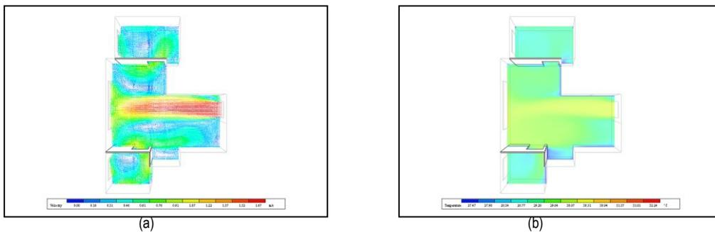
Fig. 10. (a) Air Velocity patterns (West Unit) simulation results; (b) Air Temperature Contours (West Unit)
