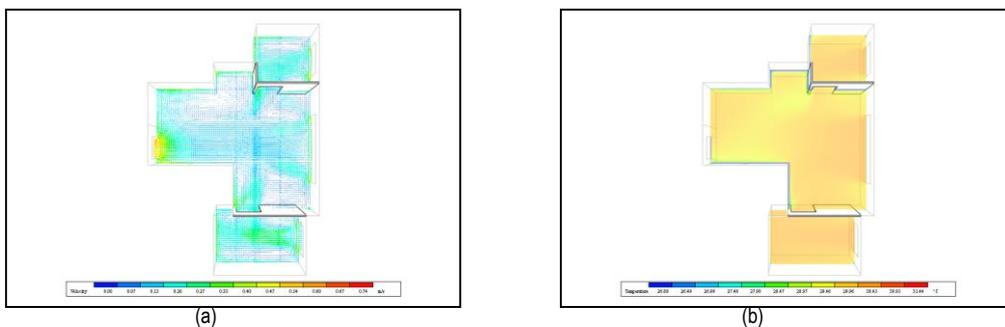
Fig. 11. (a) Air Velocity patterns (East Unit) simulation results; (b) Air Temperature Contours (East Unit)
