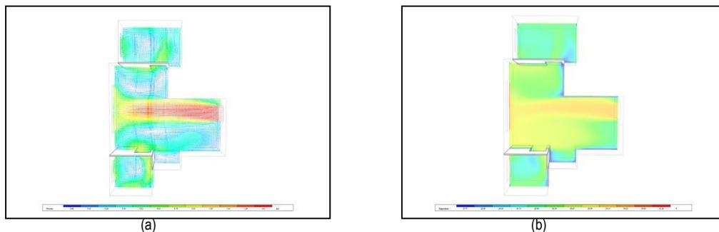
Fig. 6. (a) Air Velocity patterns (West Unit) simulation results; (b) Air Temperature Contours (West Unit)
