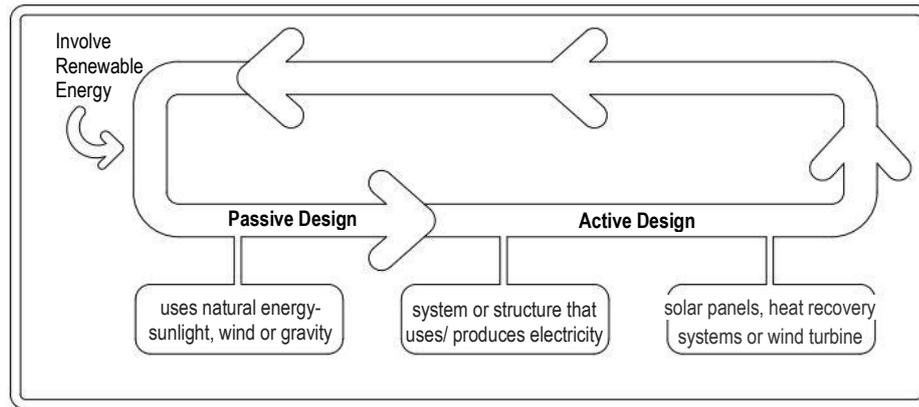
Fig. 2: The correlation between passive design and active design for low energy buildings
