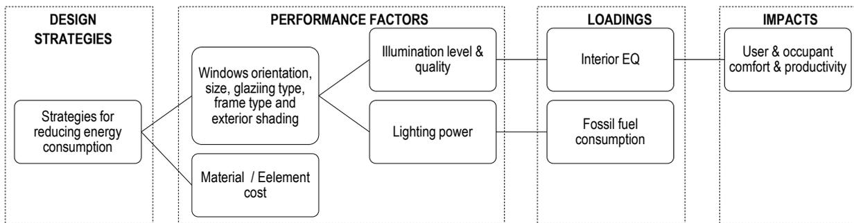
Fig. 1: The relationships between design strategies, performance factors, loadings and impacts from SB Tool rating tool (Source: SB Tool)
