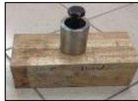
Fig. 7: Bolt inserted into the cylinder slot
