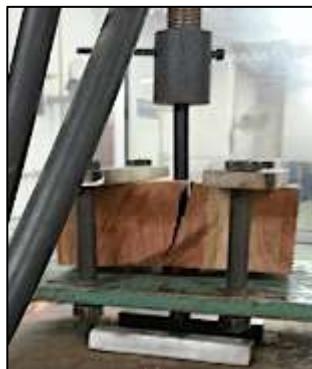
Fig. 15: Typical splitting for parallel with and without the glue line
