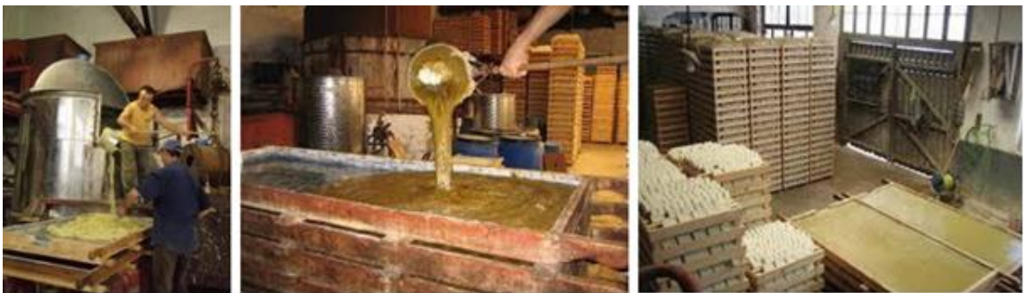
Fig. 7. Traditional Soap Industry Production Processes.
