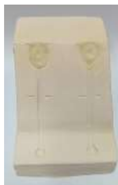
Fig. 7: The powder ball was placed into a curves shape on flow test block
