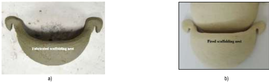
Fig. 10. (a) Fabricated scaffolding nest; (b) Fired scaffolding nest
