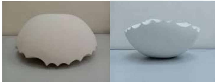
Form without setter - Warped and bottom profile change drastically
