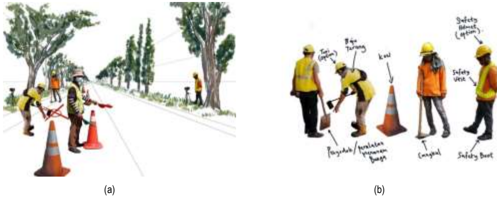
Fig. 5. (a) Process for On-Site Installation; (b) Recommended Protective Apparel During Operation. (Source : Muhammad Sukor Bin Romat)
