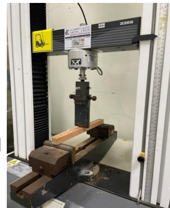
Fig. 3: (a) Schematic diagram of 3-point bending test; (b) Set up for the 3-point flexure bending test
