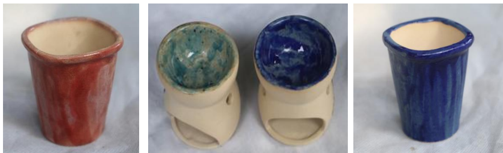
Fig 7. The result of the effect of powdered glass waste shards combined with soil and applied to ceramic products. (Source: Author's Documentation 2019)
