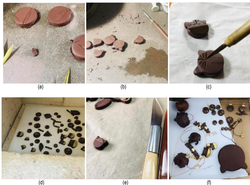
Fig. 1. (a) Cutting; (b) Shaping; (c) Gilding; (d) Re-firing; (e) polishing; (f) Install. (Source: Personal Photo Archive, 2024)
