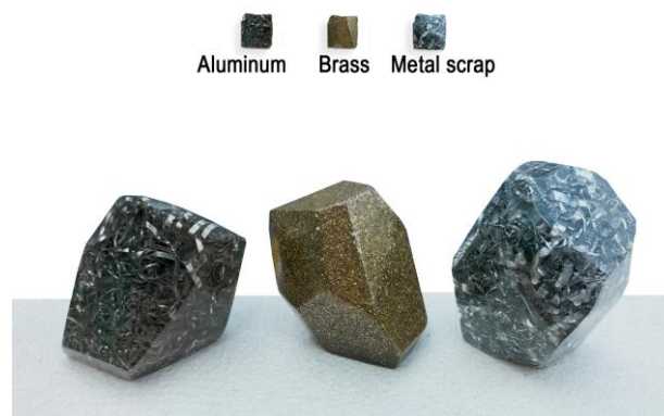
Fig. 2: The image of selected industrial toxic waste mixing with adhesive experiment results (Source:) The authors
