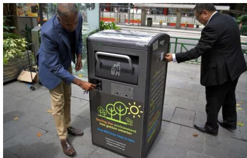
Fig. 3: BigBelly Waste bin in Singapore will send alerts for them to be cleared when they are almost complete. (Source: https://www.straitstimes.com/singapore/solar-powered-smart-bins-that-act-as-wi-fi-hotspots-launched-at-orchard-road )
