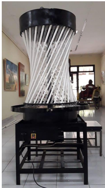
Fig. 2: Eco-art photobioreactor installation with "Vertically Twisted Spiral Lines" configuration (Source: Burhan et al., 2021).
