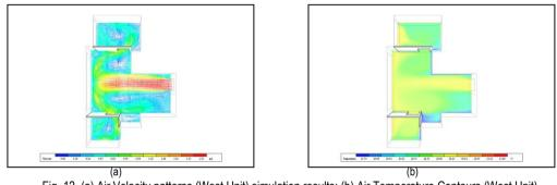
Fig. 12. (a) Air Velocity patterns (West Unit) simulation results; (b) Air Temperature Contours (West Unit) (Source: Author)
