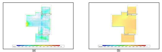
Fig. 11. (a) Air Velocity patterns (East Unit) simulation results; (b) Air Temperature Contours (East Unit) (Source: Author)
