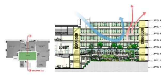
Fig. 2. Section A-A of the courtyard garden of the H1 hospital. (Source: H1 Architects. Sdn. Bhd, re-illustrated by Author 2018)
